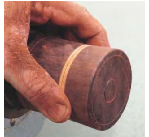
STEP 33. You can see from the state of my hand the problems of working with colourful timber: you will find that the red dust from the rosewood will contaminate the grain of the lighter wood if you use an opened-grained species
